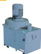
B73 Coolant Tank
